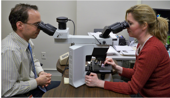
Figure 2: Common practice for collaborative diagnosis using a dual view microscope. In this workflow, one person drives the microscope while the other simultaneously watches through separate microscope oculars. Other versions of multiheaded microscopes have three or more oculars.
