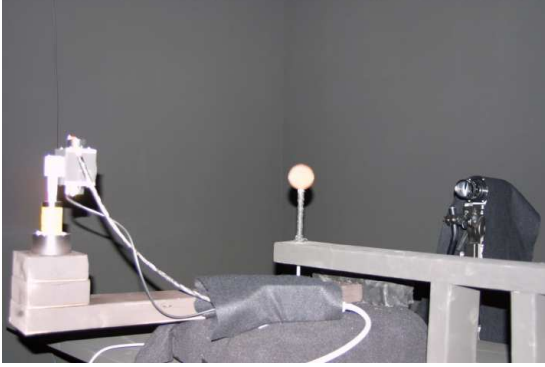
Figure 1: A photograph of our isotropic BRDF measurement device.
