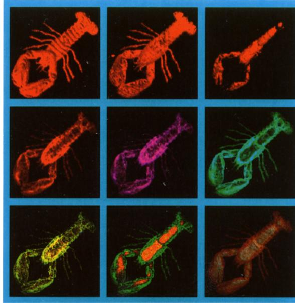
Fig. 12. Volume rendered images of a  $128^3$  dataset of a CT lobster rendered with the sub-volume implementation of Cube-4 on the Teramac. Each image took 0.6 s on the Teramac running at very low 0.96 MHz.
