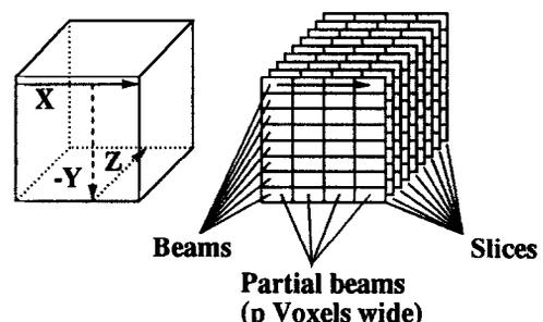
Fig. 4. Volume traversal for beam partitioned slice-parallel ray-casting.
