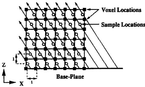
Fig. 1. Template-based ray-casting.
