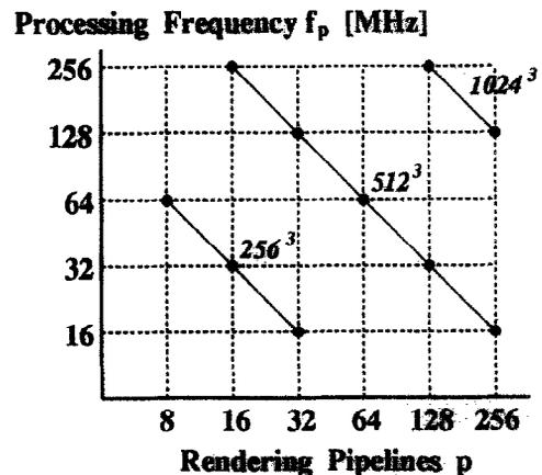
Fig. 13. Processing frequency,  $f_p$ , vs the number of rendering pipelines  $p$  for three dataset resolutions. Rendering performance is  $f_r = 32$  frames per second.
