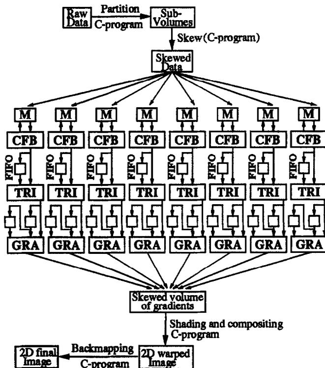
Fig. 9. Block diagram of the sub-volume partitioned Cube-4 implementation on the Teramac with eight rendering pipelines (M, DRAM Memory Module; CFB, Cubic Frame Buffer Address Generation; TRI, Tri-linear Interpolation Unit; GRA, ABC Gradient Estimation Unit).
