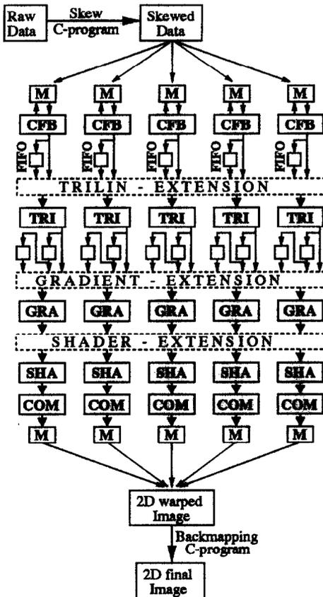
Fig. 10. Block diagram of the beam partitioned Cube-4 implementation on the Teramac with five rendering pipelines (M, DRAM Memory Module; CFB, Cubic Frame Buffer Address Generation; TRI, Tri-linear Interpolation Unit; GRA, ABC Gradient Estimation Unit; SHA, Shading Unit; COM, Compositing Unit). The interconnections provided inside the extension units are only local, not global.
