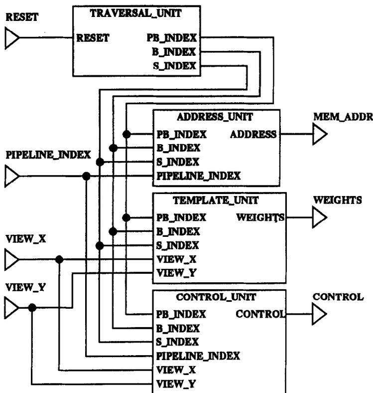
Fig. 11. CFB address unit block diagram. *PB\_INDEX* indicates the index of the current partial beam, while *B\_INDEX* and *S\_INDEX* indicate the current beam and slice-index.
