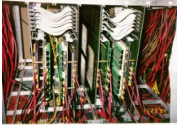
Fig. 6. Four Teramac boards, connected to each other with ribbon cable, and to a controller board. The pins of one multi-chip module (MCM) can be seen in the middle.
