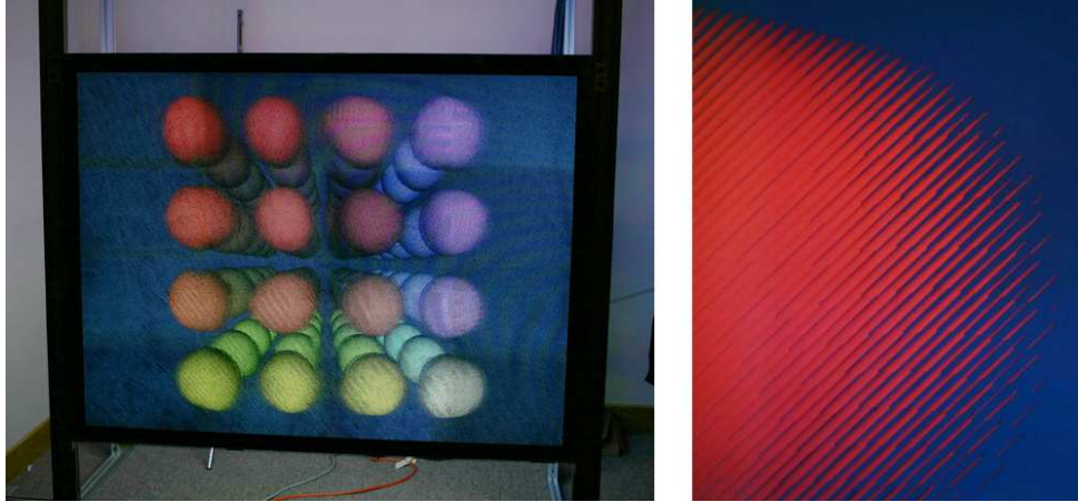
Figure 7. Left: Physical setup of the software multiplexing display. Right: Close-up of high resolution image with multiplexed views.
