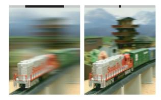
Figure 9: Simulated display views without depth compression (left) and with depth compression (right). We map the locomotive into the depth of field of the display, which reduces the maximum display disparity from 206 to 10 pixels.
