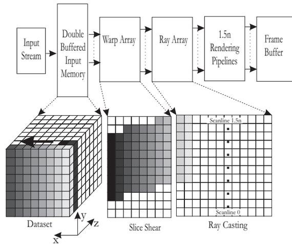
Figure 6: *Array Based Ray Casting architecture.*
