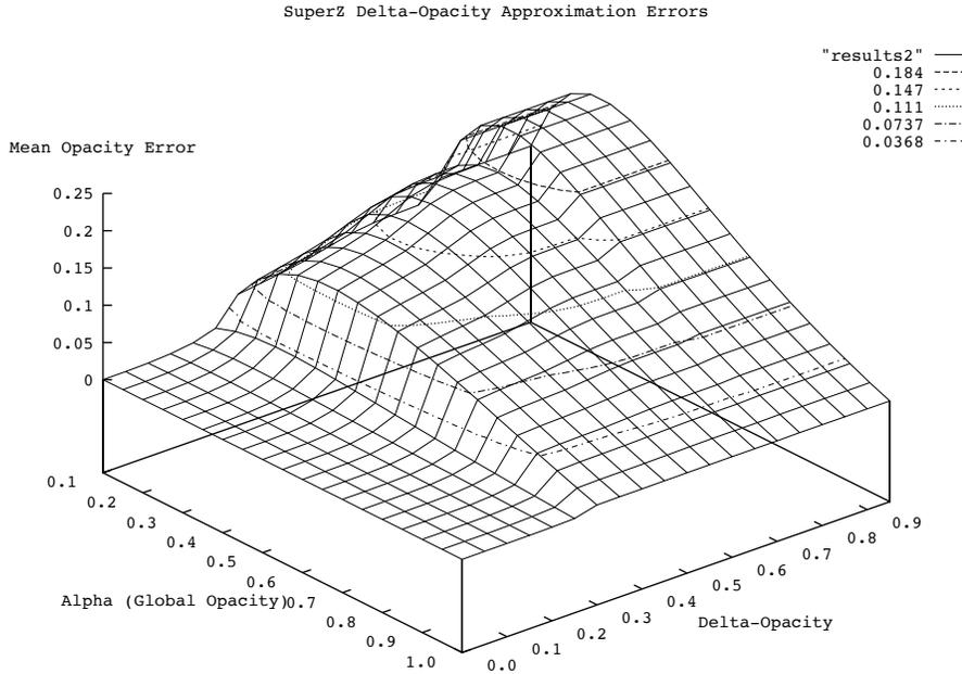
**Figure 11.** The variation in mean opacity error against global opacity  $t$  at different approximations ( $\delta$ ). The comparison was made against a full ray cast image. The error increases both with the degree of compositing approximation used ( $\delta > 0$ ) and lower object opacity.
