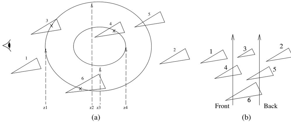
**Figure 27.** (a) Possible triangle positions rendered within an example volumetric scene. Types 1 and 2 lie in front and behind all voxel data. Triangle types 3 and 4 intersect surfaces of volume data. Type 5 intersects a “backface” and will be treated the same as type 2. Type 6 intersects the surface of a volume and straddles two clipping planes. (b) Triangle types clipped against a pair of depth planes. Types 1 and 2 are not sent. Types 3, 4, 5 and 6 are rasterized.
