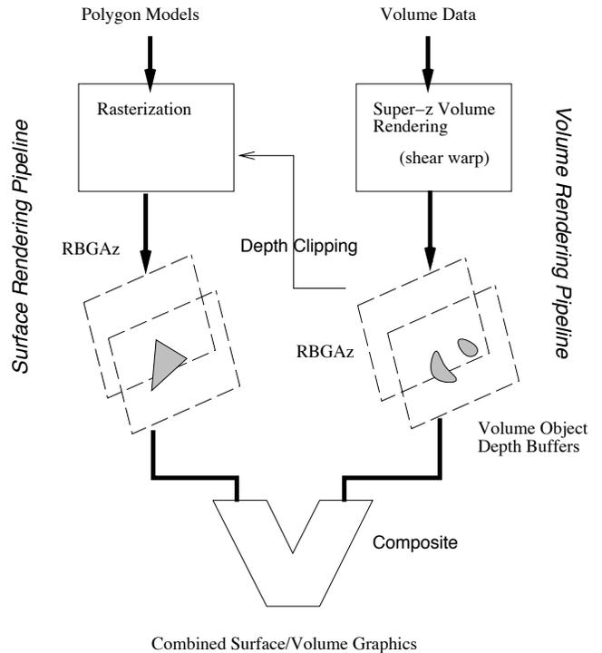
Figure 5. Mixing surface geometry and volume rendered graphics using super- $z$  depth buffering. Polygon rasterization is controlled by the depth buffering. Polygon pixels and volume segment pixels are composited in an interleaved fashion by arithmetic and logic in the compositor.
