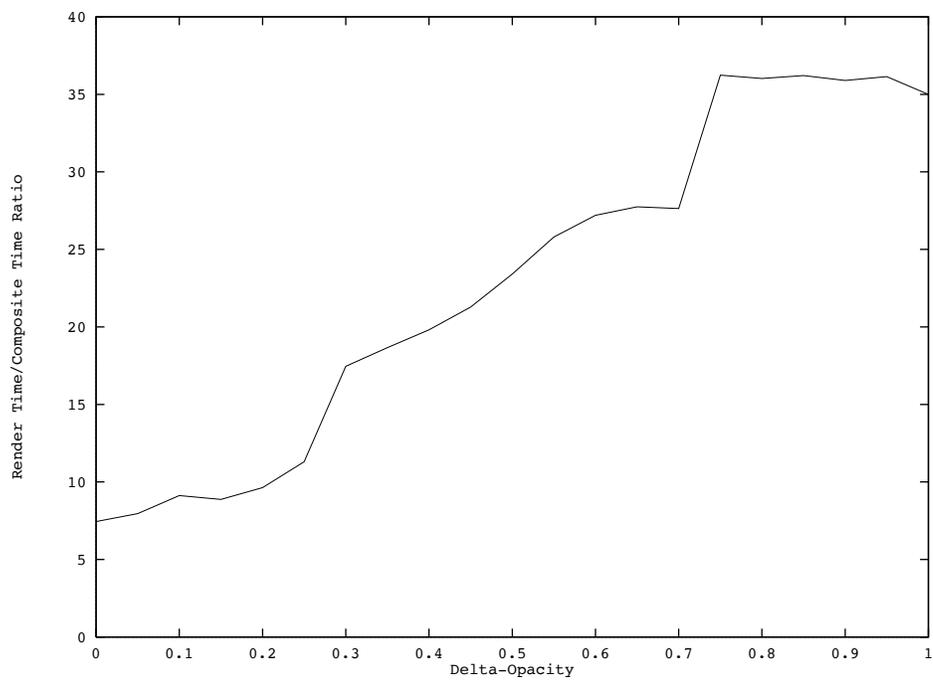
**Figure 32.** Plot showing effect of various opacity approximation thresholds ( $\delta$ -Opacity) against ratio of Render/Composite time. The best Render/Composite ratios are at low approximation thresholds. The relationship is roughly linear ranging from 7 times to 35 times faster compositing.
