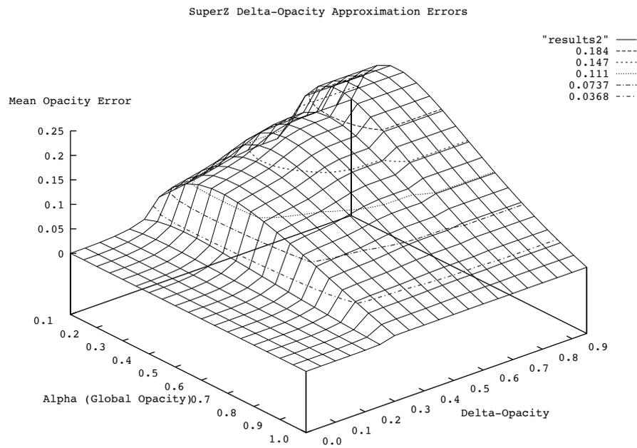
**Figure 29.** The variation in mean opacity error against global opacity  $t$  at different approximations ( $\delta$ ). The comparison was made against a full ray cast image. The error increases both with the degree of compositing approximation used ( $\delta > 0$ ) and lower object opacity.
