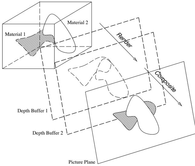
**Figure 19.** Overview of depth buffer volume rendering
