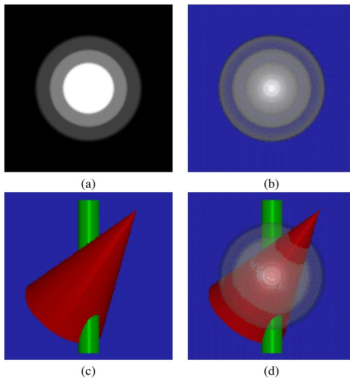
**Figure 28.** Synthetic volume and geometry data used for opacity error quantification. (a) Cross-section through the concentric spheres volume data. (b) Full ray-cast of (a) at global opacity 0.5. (c) Geometry data consisting of a cylindrical bar and cone. (d) Intermixed volume and geometry (volume opacity 0.5).
