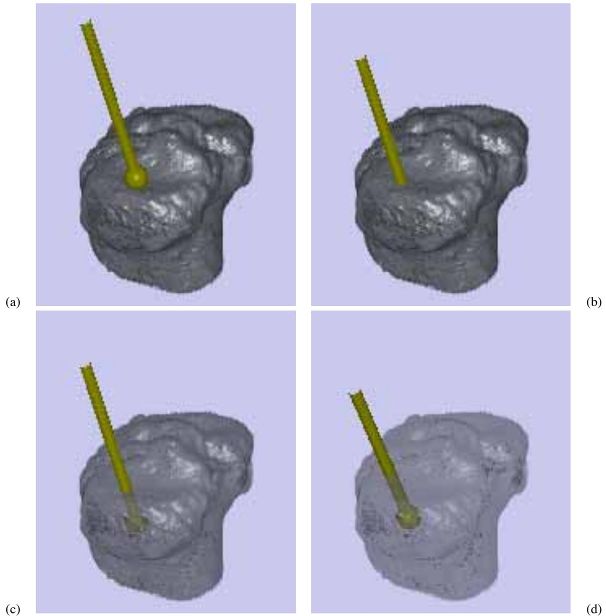
**Figure 18.** Four frames from a simulated haptic probing of the surface of a volume rendered tibia from the knee joint data set. The probe is represented by a polygonal cylinder and sphere (1160 polygons), separately rendered by polygon accelerated frame graphics. Super-z is used to combine the renderings as the probe is moved and breaks the tibial surface. In (d) transparency of the bone was reduced to show the probe inside the bone.
