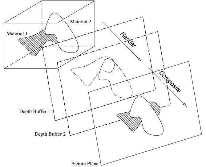
Figure 1. Overview of depth buffer volume rendering
