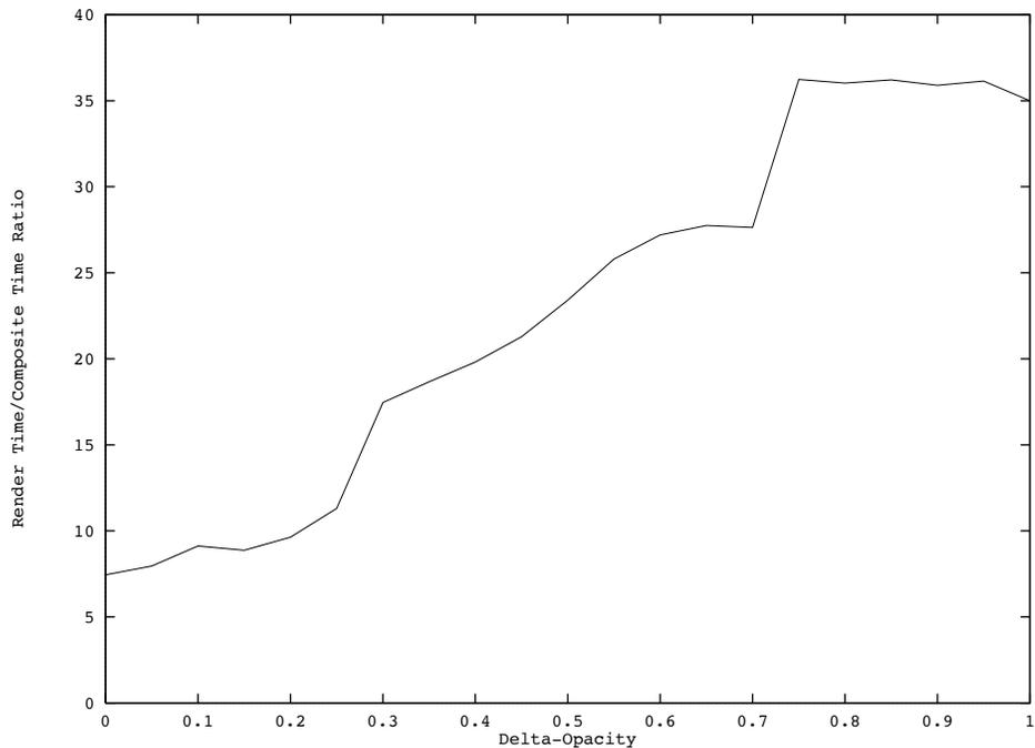
**Figure 14.** Plot showing effect of various opacity approximation thresholds ( $\delta$ -Opacity) against ratio of Render/Composite time. The best Render/Composite ratios are at low approximation thresholds. The relationship is roughly linear ranging from 7 times to 35 times faster compositing.
