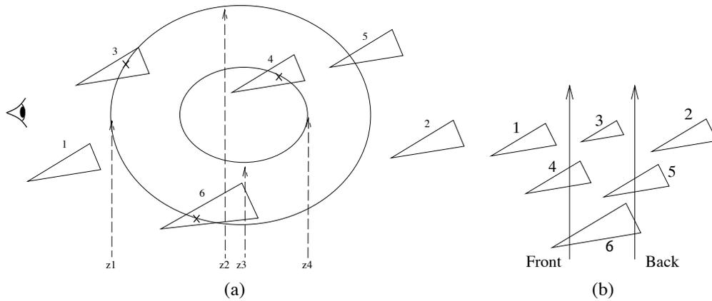
**Figure 9.** (a) Possible triangle positions rendered within an example volumetric scene. Types 1 and 2 lie in front and behind all voxel data. Triangle types 3 and 4 intersect surfaces of volume data. Type 5 intersects a “backface” and will be treated the same as type 2. Type 6 intersects the surface of a volume and straddles two clipping planes. (b) Triangle types clipped against a pair of depth planes. Types 1 and 2 are not sent. Types 3, 4, 5 and 6 are rasterized.
