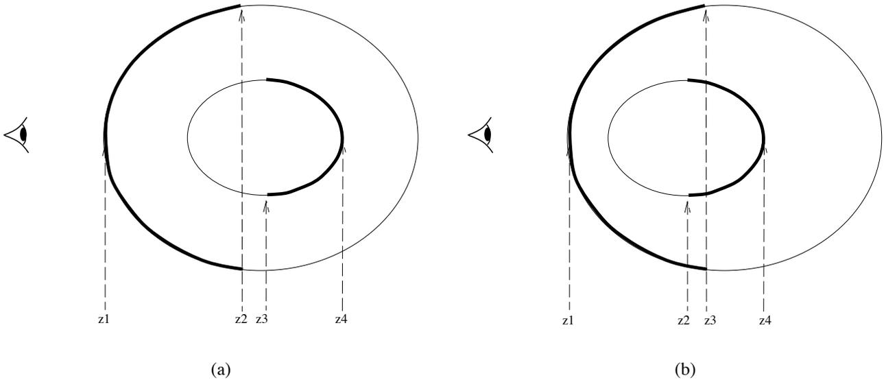
**Figure 8.** Min-max segment values and depth hulls for torus shaped volumes seen side on. In (b) the inner hull overlaps the outer hull and  $z_2$  and  $z_3$  planes are reversed in comparison to (a).
