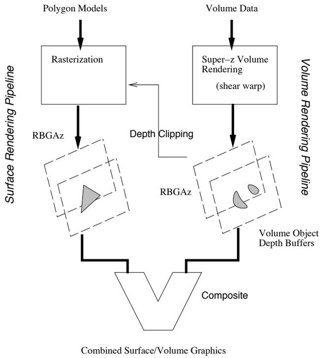
**Figure 23.** Mixing surface geometry and volume rendered graphics using super-z depth buffering. Polygon rasterization is controlled by the depth buffering. Polygon pixels and volume segment pixels are composited in an interleaved fashion by arithmetic and logic in the compositor.
