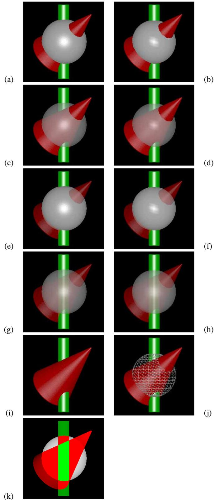
**Figure 15.** Left column: super-z volume renderings of synthetic volumes: sphere, cone and cylindrical bar. Right column: combined volume-geometry using super-z, with sphere polygon rendered. In (j) the wireframe (1200 triangles) defining the sphere is shown. In (k), where objects overlap the following color coding is used: red, green, blue, yellow, cyan, magenta, for overlaps of 1, 2, 3, 4, 5 and 6; and white for overlaps of greater than 6.
