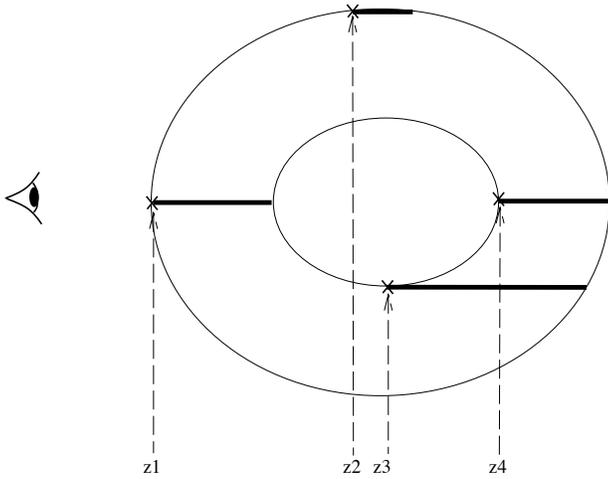
**Figure 7.** Minimum and maximum segment start depth values for a simple torus shaped volume are at:  $z[1,2]$  for the first segment of all rays, and  $z[3,4]$  for the second segment. Therefore,  $z[1,2,3,4]$  define depth planes used to control the order of polygon rasterization. The pseudo planes  $z = 0$  and  $z = \infty$  are added to this list.
