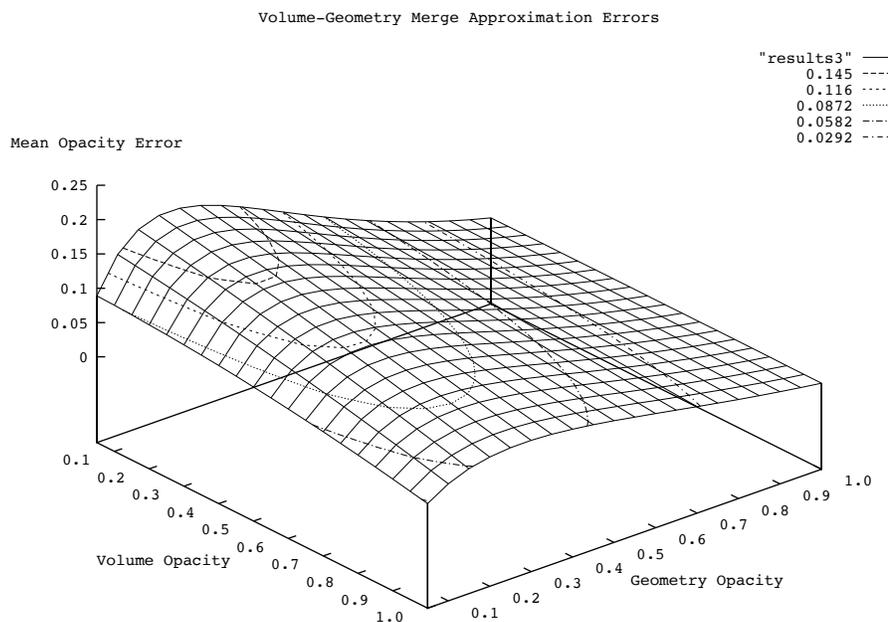
**Figure 12.** The variation in mean opacity error for different volume-geometry opacities for  $\delta = 1.0$  (zeroth order super-z). The comparison was made against a full ray cast image. The error minimizes with increasing volume and geometry opacity i.e. the more solid are the objects. The error peaks at a geometry opacity of around 0.3. The effect of the volume opacity on the overall error is fairly linear.
