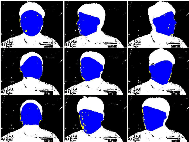
Figure 9: Shape fitting for a monocular sequence (white is input, yellow is the model, and blue is model-input intersection).
