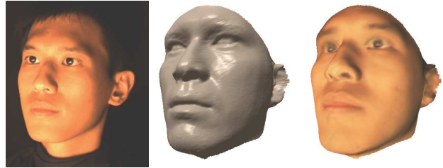
Figure 7: A rendering of the captured 3D model of an Asian subject. Left panel is a (real) image taken from our rig. Note: subject was not laser-scanned or included in the training set.
