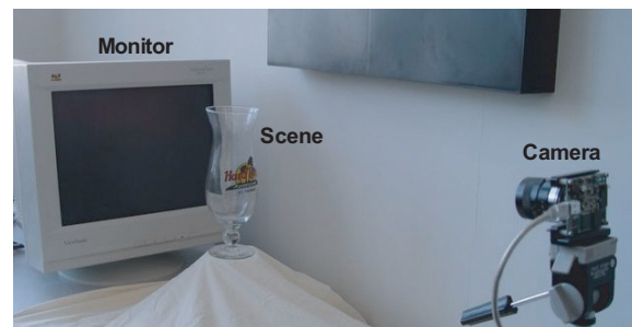
Figure 4: Acquisition system for indoor scenes.
