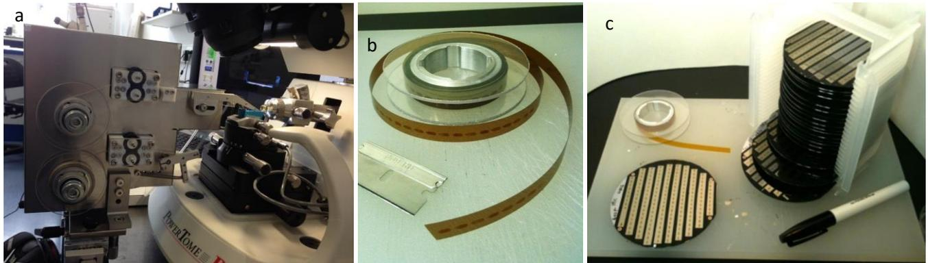
**Figure 1.** (a) ATUMtome used to collect 30 nm thick serial sections. (b) a typical reel of tape with sections (dark rectangles) collected on tape. (c) library of wafers containing thousands of serial sections.
