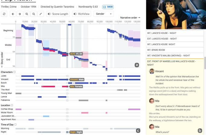
Fig. 2. Overview of Story Explorer with three embedded views: (a) story curve view, (b) script view, and (c) metadata view. The story curve succinctly summarizes the nonlinear narrative of *Pulp Fiction* with additional metadata displayed along the story curve.
