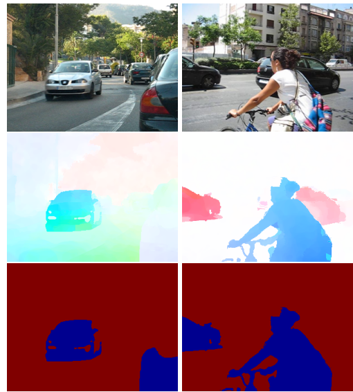
Figure 9. Motion estimation and segmentation results on the MIT benchmark. From top to bottom: First frame of video; Flow estimate; Segmentation. The fully connected layered model can recover the fine structures in the scene, such as the background holes in “Car3” (right column).
