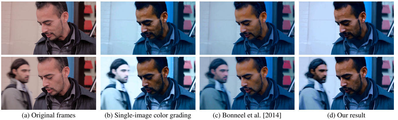
Figure 6: Bonneel et al. [2013] introduced a single-image color transformation model, which when applied per frame, produces temporal inconsistencies (see brightening in the background) (b). They eliminate this inconsistency by filtering color-transforms in a higher-dimensional space (c); we achieve a similar consistency with our algorithm that is blind to the color transfer (d).
