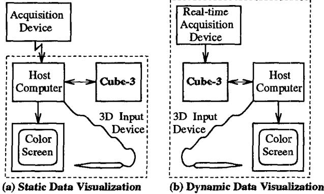
Figure 1: Real-Time Volume Visualization Systems.
