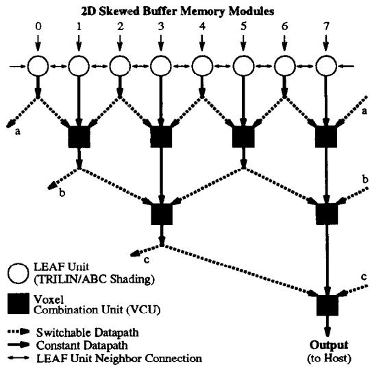
Figure 7: Folded Binary Cone Tree ( $n = 8$  Leaf Nodes).
