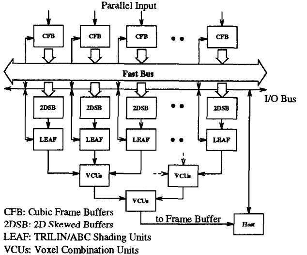
Figure 8: Cube-3 Hardware Architecture.
