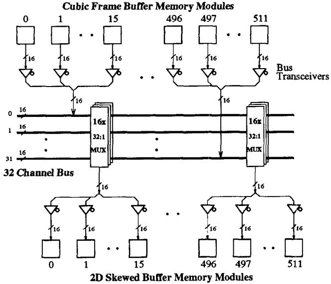
Figure 4: Fast Bus Configuration for  $n = 512$ .
