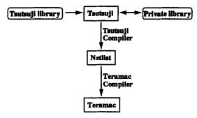
Fig. 8. Design-flow for Teramac.
