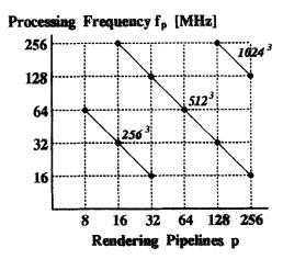
Fig. 13. Processing frequency,  $f_p$ , vs the number of rendering pipelines p for three dataset resolutions. Rendering performance is  $f_r = 32$  frames per second.
