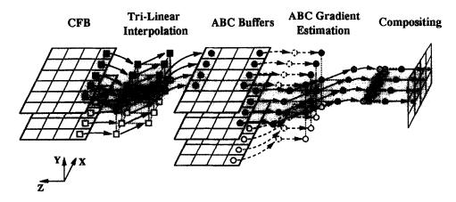
Fig. 2. Dataflow of slice-parallel ray-casting (CFB, Cubic Frame Buffer; ABC, Above Below Current).
