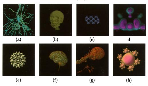
Fig. 14. Volume rendering images of 128<sup>3</sup> datasets produced by the beam partitioned implementation of Cube-4 on Teramac. Each image took 1.5 s at very low 0.2 MHz clock rate. (a) Hippocampal pyramidal cell. (b) CT head, 45° rotated. (c) Simulated silicon lattice. (d) Simulated high-potential iron protein. (e) Volume-sampled geometric mechanical part. (f) MRI brain. (g) Bullfrog ganglion cell. (h) Volume-sampled sphere flake.
