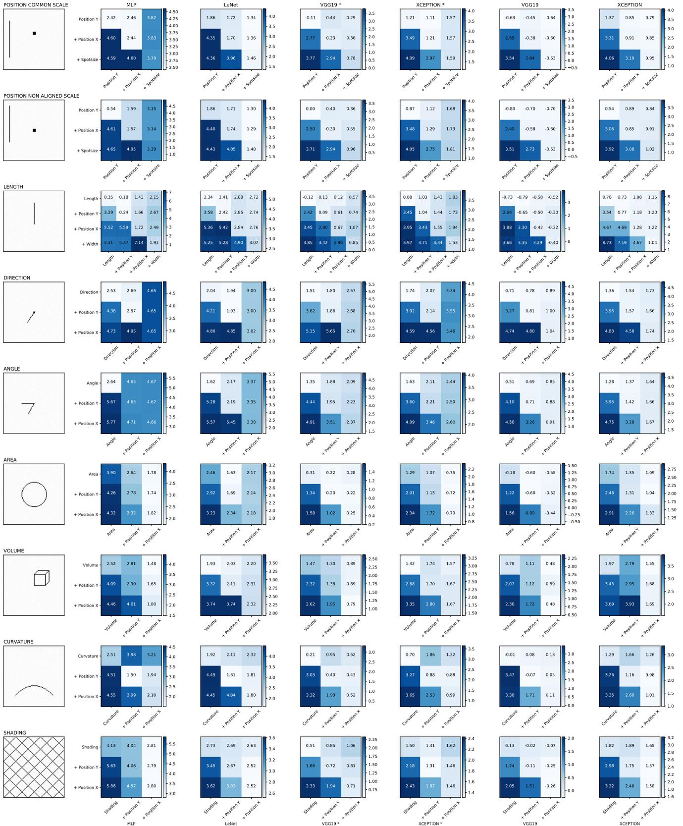
Fig. 9: **Cross-network variability.** Our networks fail when the stimuli changes through translation or stroke width. The x-labels indicate the training configuration while the y-labels indicate the stimuli variation. Numbers represent MLAE.
