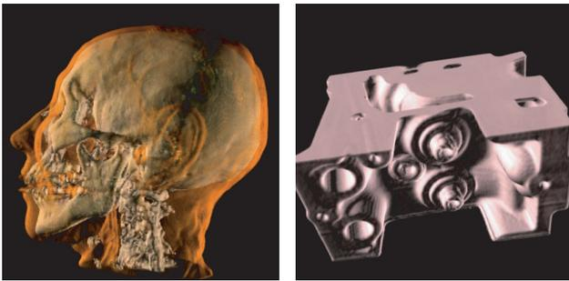
Figure 21: CT scan of a human head ( $256^2 \times 225$ ) and of an engine ( $256^2 \times 110$ ) rendered with hardware-accelerated EWA volume splatting on a GeForce FX Ultra 5900. Image courtesy of Wei Chen, Zhejiang University, China, and Liu Ren, Carnegie Mellon University, USA.
