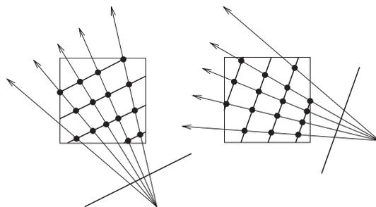
Figure 7: Image-aligned 3D texture slicing.
