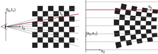
Figure 2: Transforming the volume from camera to ray space. Left: camera space. Right: ray space.
