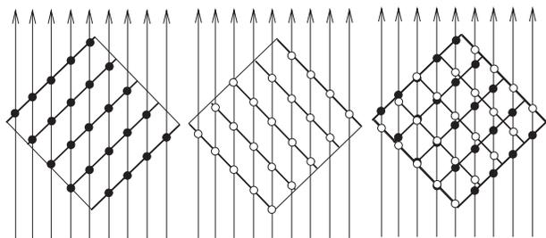
Figure 13: *Popping artifacts in 2D texture slicing. The samples along rays may not be aligned after a small change in viewing angle leads to a change of slicing direction. The superposition on the right shows that the location of resampling locations abruptly changes, which leads to sudden changes in pixel intensity. Figure suggested by Christof Rezk-Salama, University of Erlangen, Germany.*
