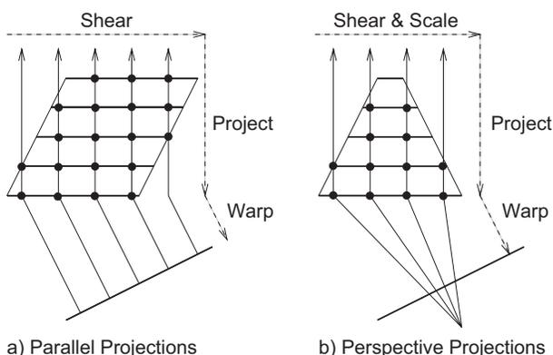
Figure 14: *Shear-warp factorization.*
