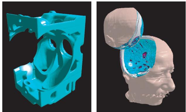
Figure 9: *Volume clipping applied to a CT scan of an engine* (left,  $256^2 \times 110$ ) and an MRI scan of a human head (right,  $256^3$ ). The cutting surfaces are enhanced by combining surface-based and volumetric shading. Image courtesy of Daniel Weiskopf, University of Stuttgart, Germany.
