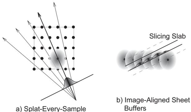
Figure 20: *Splatting algorithm*. Left: 3D reconstruction kernels are integrated into 2D footprints, projected, and composited onto the image plane. Right: Image-aligned sheet buffers slice through the kernels. The contributions of 3D reconstruction kernels within a slab are added. The result of each slab is then composited onto the image plane.
