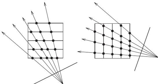
Figure 10: *Object-aligned 2D texture slicing.*
