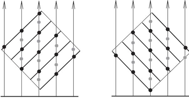
Figure 16: *Shear-image order* ray casting. Grey samples are interpolated inbetween original volume slices.
