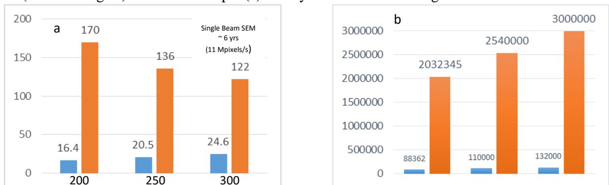
**Figure 2.** (a) the number of terabytes per day at 200, 250 and 300 Mpixels/s (blue), the number of imaging days (orange). (b) approximate number of files generated per hour (blue) and per day (orange).
