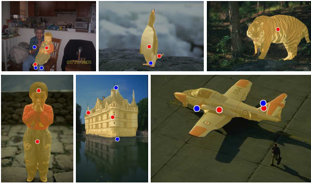
Figure 8. Segmentation results of the proposed algorithm. The segmented object masks are highlighted in yellow masks. Foreground and background user-annotations are depicted in red and blue dots, respectively.
