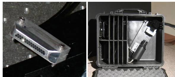
Figure 5: Left: A picture of the sensor head with linear fiber array. The source fiber is lit. Right: The fiber array leads to a camera in a light-proof box. The box is cooled to minimize imaging sensor noise.
