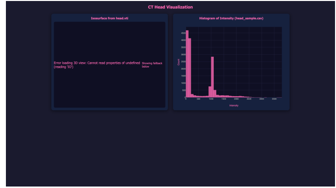
Fig. 10: Case 73 output from Claude: the isosurface panel renders only an empty container, while the pink intensity histogram is fully correct.
