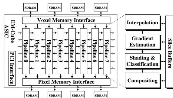
Figure 7: EM-Cube architecture with eight identical ray casting pipelines.
