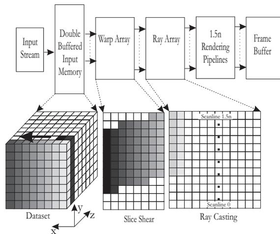
Figure 6: *Array Based Ray Casting architecture.*
