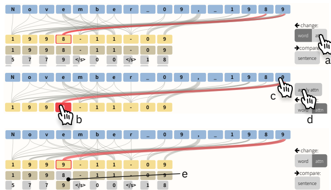
Fig. 8. To re-direct attention in Seq2Seq-Vis, the user first observes a split of attention between the input 8 and 9 for converting the last digits of a year in a date conversion model. She can (a) select attention mode, (b) select the decoder word, (c) click on the preferred encoder word, (d) apply the attention change, and (e) see the models reaction.
